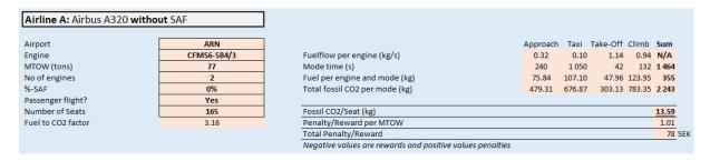
Airline B operates with an identical aircraft but uses SAF at a 20 % blend in. Airlines B is initially invoiced the same penalty, 78 SEK, however the effect of the SAF is adjusted for retroactively upon completion of the SAF-reporting. The total effect of the adjustment is then 78 - (-42) = 120 SEK in order to include re-payment of the amount initially invoiced and apply the adjusted performance.
